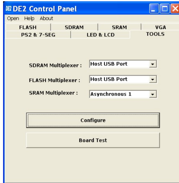
Figure 3.10. Use the Asynchronous Port 1 to access the image data in the SRAM.
